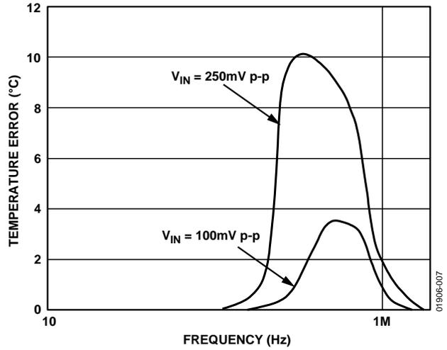
Figure 7. Temperature Error vs. Power Supply Noise Frequency
