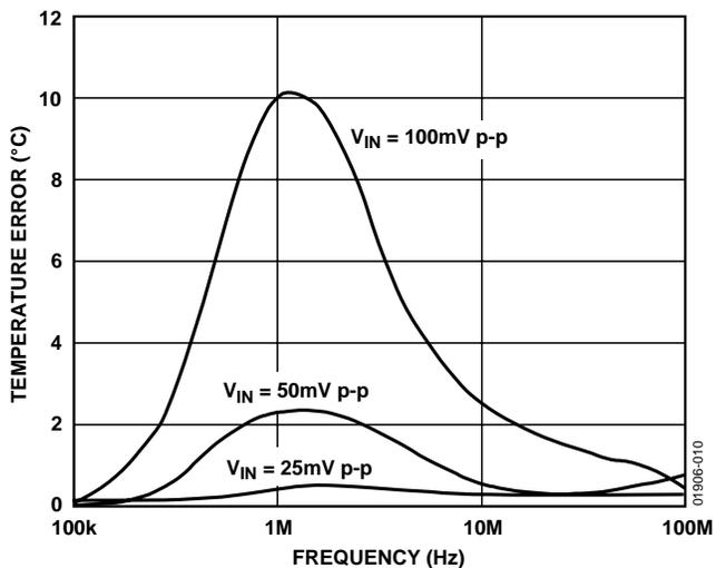
Figure 10. Temperature Error vs. Common-Mode Noise Frequency
