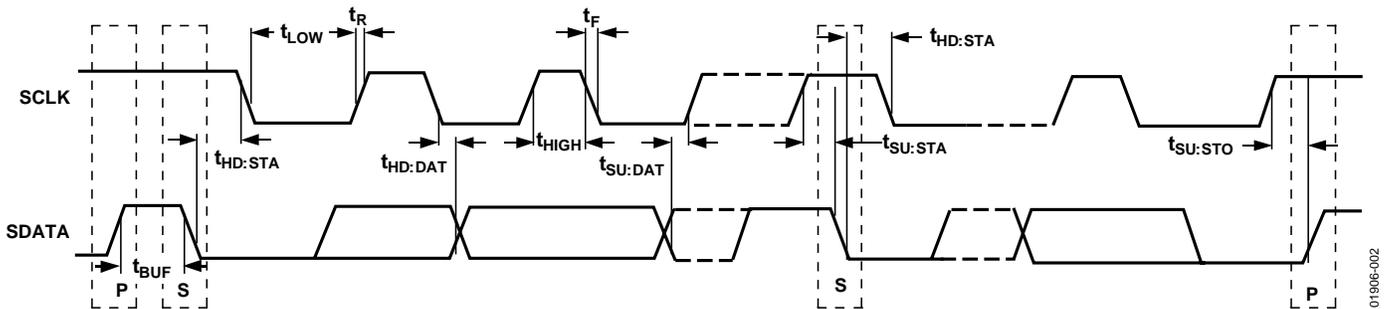
Figure 2. Diagram for Serial Bus Timing
