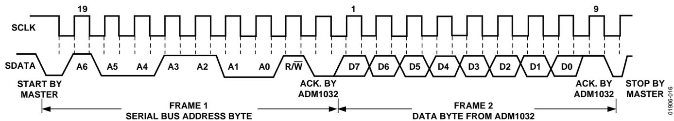
Figure 16. Reading Data from a Previously Selected Register
