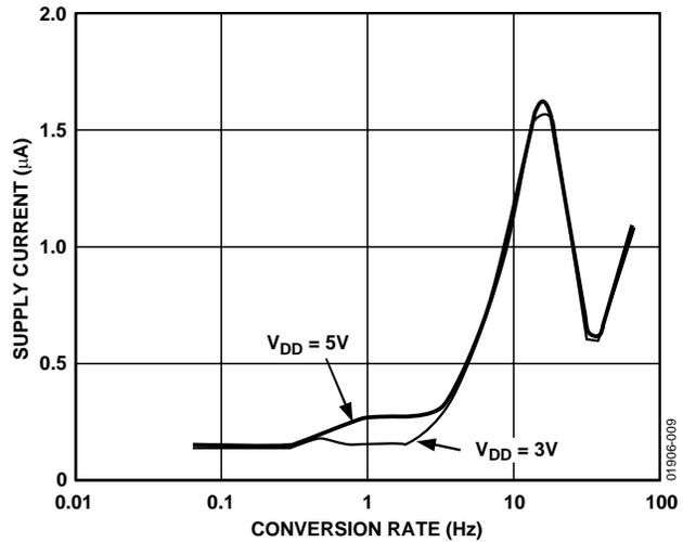
Figure 9. Operating Supply Current vs. Conversion Rate
