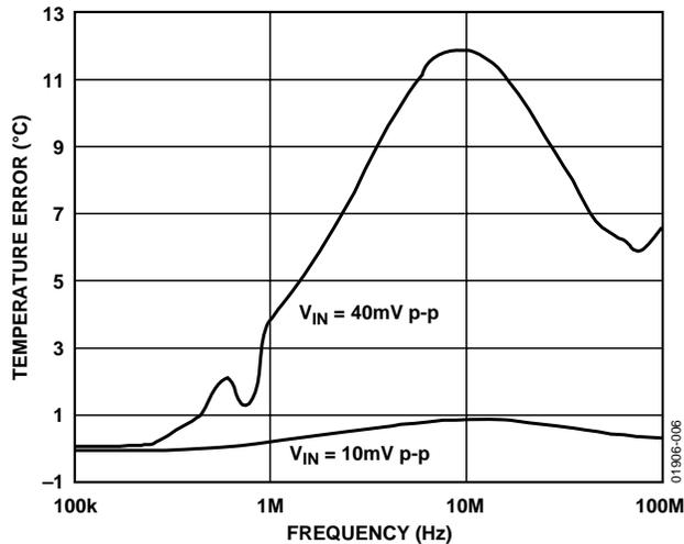
Figure 6. Temperature Error vs. Differential Mode Noise Frequency
