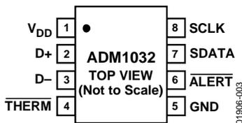
Figure 3. Pin Configuration
