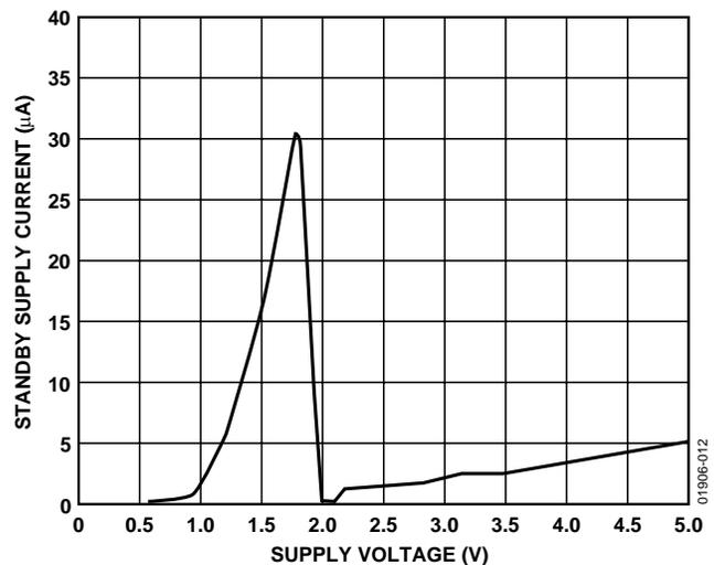
Figure 12. Standby Supply Current vs. Supply Voltage
