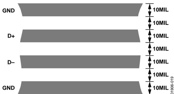
Figure 19. Arrangement of Signal Tracks
