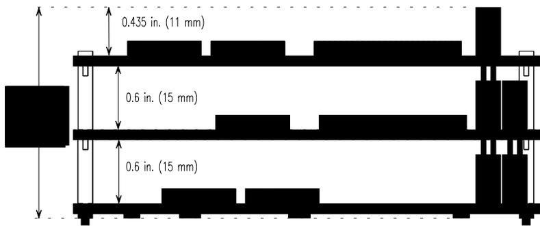
**Figure 1. Typical Module Stack**
