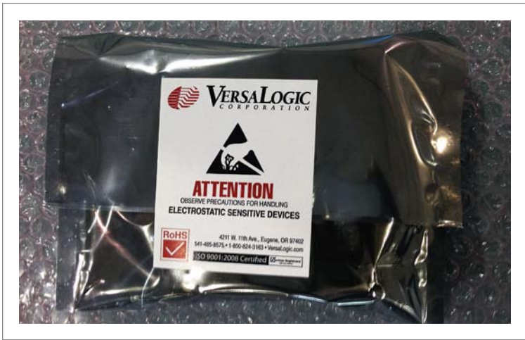
Proper packaging of static sensitive product. The sensitive board is sealed in a nickel coated static shield bag.
