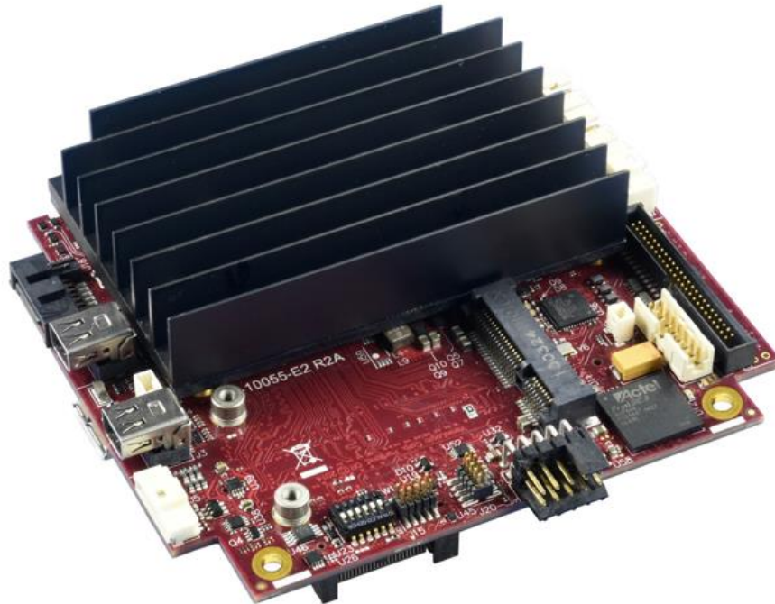
Figure 21. Installing the Passive Heat Sink
