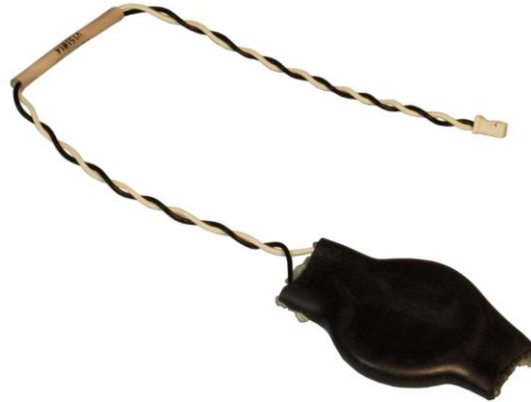
Figure 14. VL-CBR-0203 Latching Battery Module
