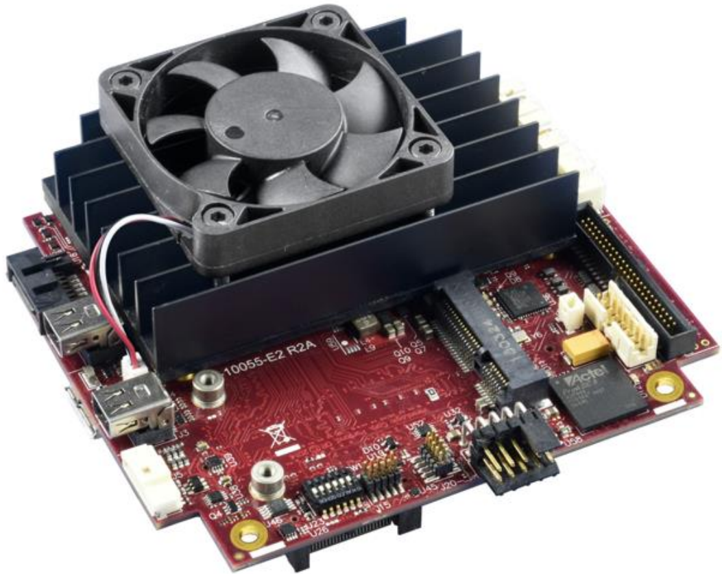
Figure 22. Installing the Heat Sink Fan
