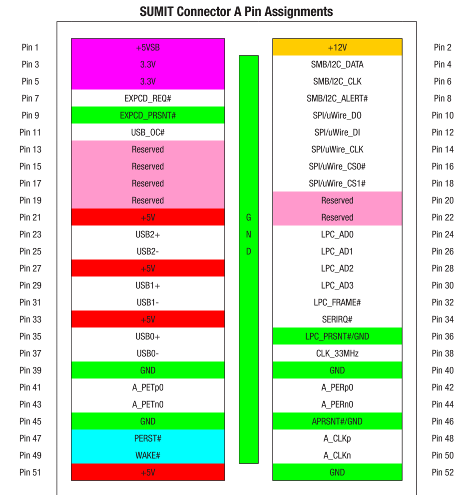
Figure 2a Detailed pin definitions for SUMIT connector A.
